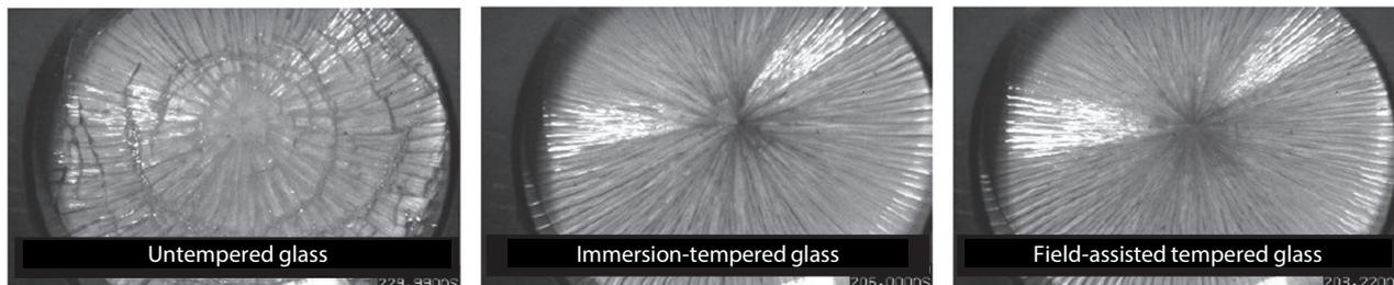
Fig. 6 Fracture of Each Glass
