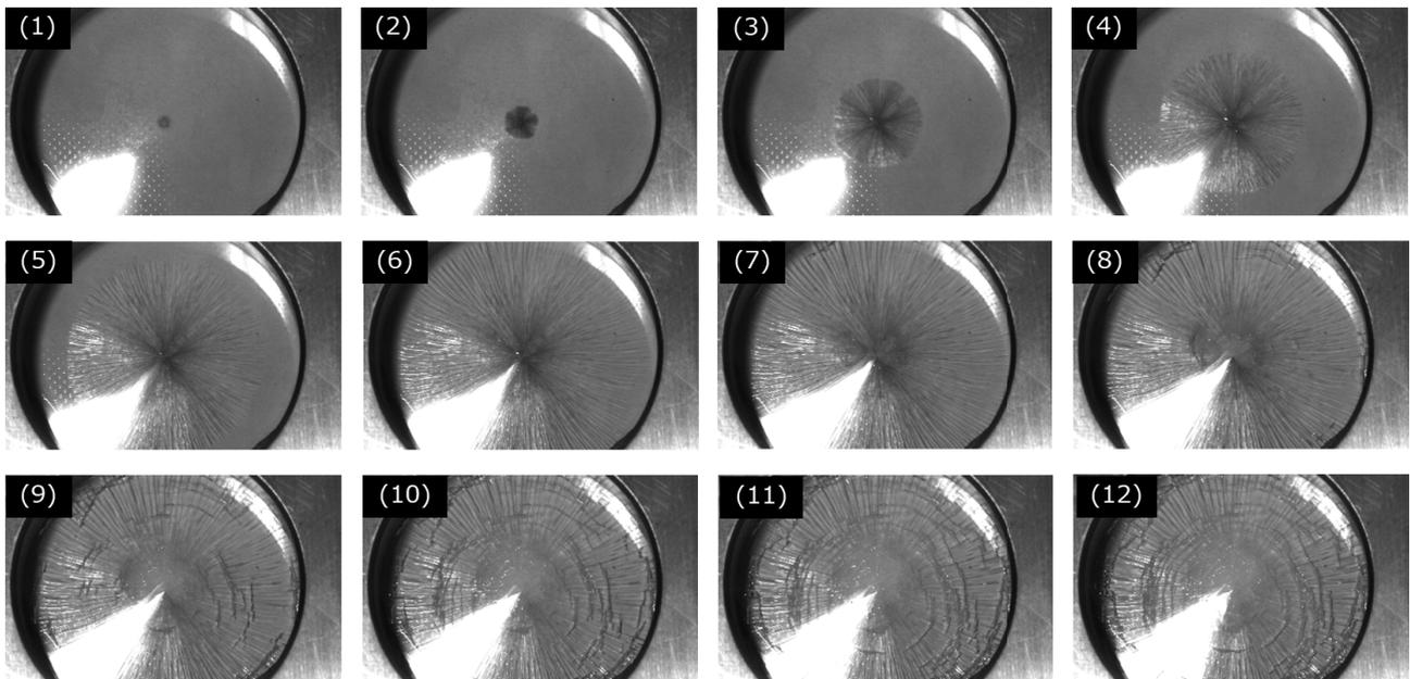
Fig. 4 Fracture of Field-Assisted Tempered Glass (time interval between images: 500 ns)
