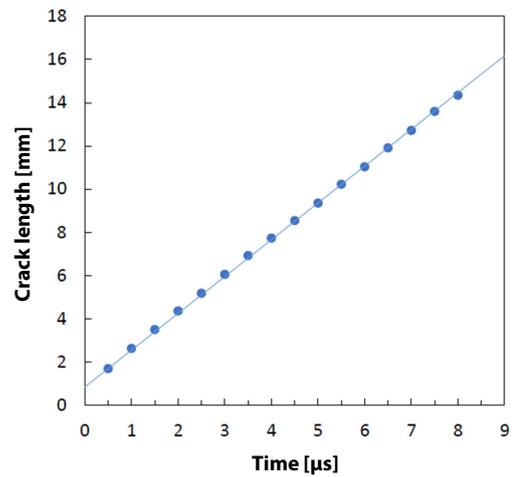
Fig. 5 Crack Length and Time in Field-Assisted Tempered Glass
